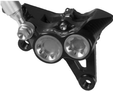
**The Mono M4 caliper** - A caliper with 4 pistons. The caliper is anodised black with "mono m4" etched onto the back of the caliper. Two caps are screwed into the front of the caliper. The caliper number is etched onto the back of the lower mounting bracket. Open system. This caliper must be used with a Mini lever. 180mm front caliper shown.
